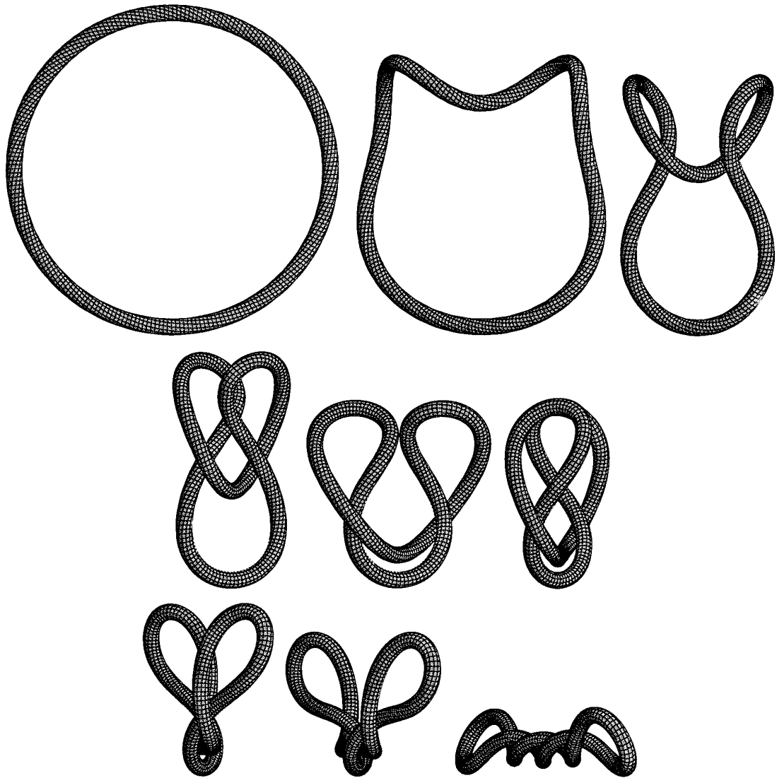
FIG. 5. Approach to equilibrium “plectonemic” conformation. First row: t = 0 , t = 0.35 , t = 0.45 . Second row: t = 0.55 , t = 0.75 , t = 0.95 . Third row: t = 1.25 , t = 1.55 , t = 3.50 .
